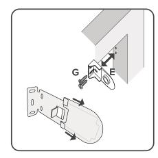
Slide bracket cover off to expose screw holes. Discard Cover. Secure inside window frame as shown above using screws provided.
