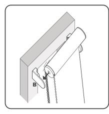
Insert chain mechanism **(C)** into the desired side of roller tube. Insert idler end **(D)** into the opposite end.
