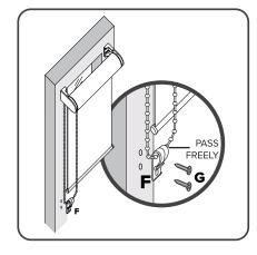
Lightly tension ball chain and fit tension device securely to architrave/wall. Allow enough play for chain to pass through device freely.
