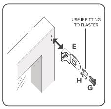
Secure to Architrave or Wall as shown above using screws provided. Use plaster plugs if fixing to wall.
