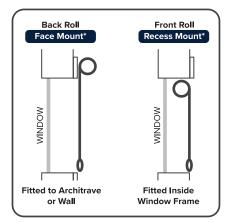
Fabric can be rolled from the front or back by simply flipping the entire roller tube or re-rolling the blind backwards.
