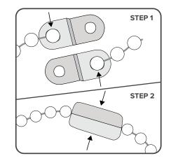
To shorten current roller blind chain: • Cut excess chain using scissors\* • Place the last bead from the chain into the ball slot of one half of the chain joiner • Repeat for the other half of chain joiner • Clip the two halves together, you should
