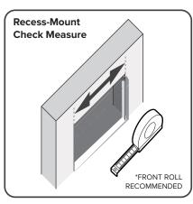
Recess Mounted blinds are fixed inside the window frame. Measure width to fill opening as shown above.
